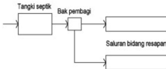
Gambar 6. Sistem Resapan (SNI 2398-2017)
